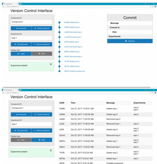
Figure 11: Screenshot of web interface. Shows two ways of displaying the compound versions: source tree (top) and table (bottom).
